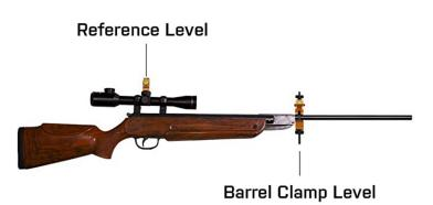
Attention the placement of the reference level on a wide, flat area that is level with the receiver and that the level itself sits perpendicular to the rifle bore.
